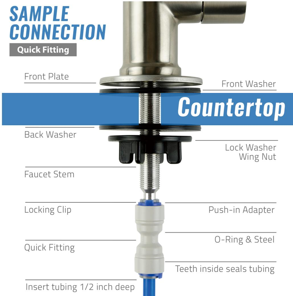
**2.** Slide the front plate and front washer onto the faucet stem. Insert the faucet stem into the hole on the countertop. Under the sink, insert back washer and tighten the wing nut (you may apply a few rounds of Teflon tape to the threads to get a better grip).
